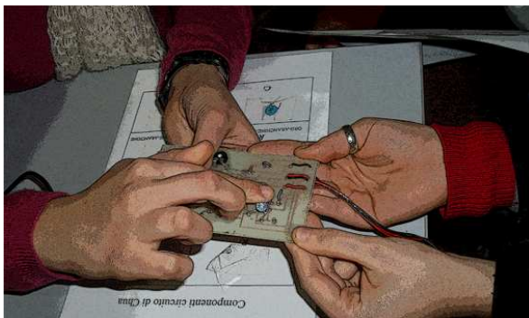
Figure 6. Construction of the Chua's circuit
